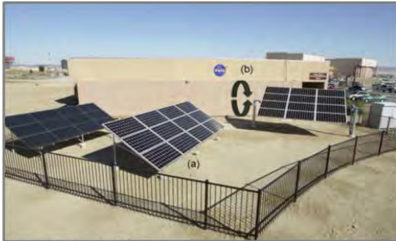
Figure 2.6: (a) Fixed axis tracking system and (b) single axis tracking system (Source: Mulilo Renewable Project Developments)
