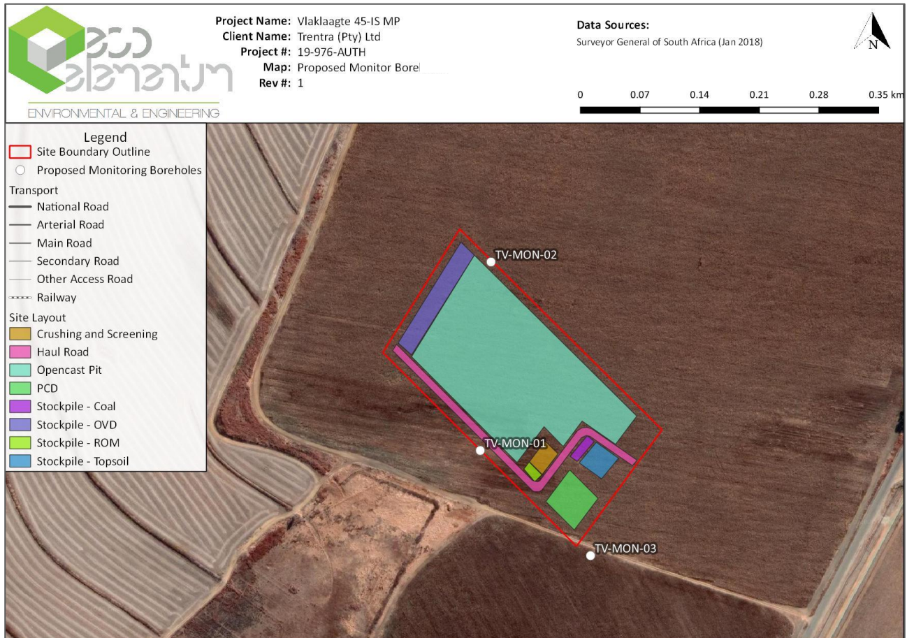
Figure 22: Positions of the monitoring boreholes to form part of the monitoring program at Trentra Vlaklaagte mining.
