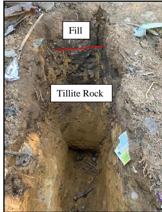
Plate 7: Fill and tillite rock at IP16
