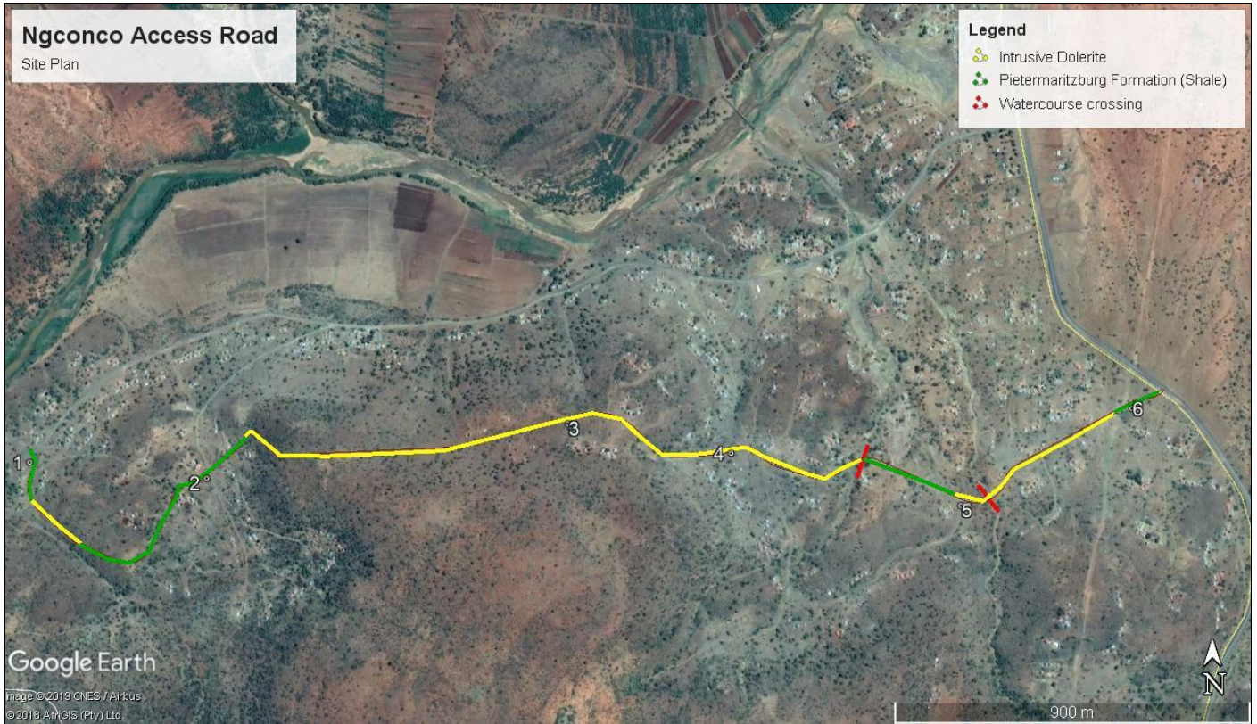
Figure 2: Site Plan with areas underlain by shale (green) and dolerite (yellow) indicated.
