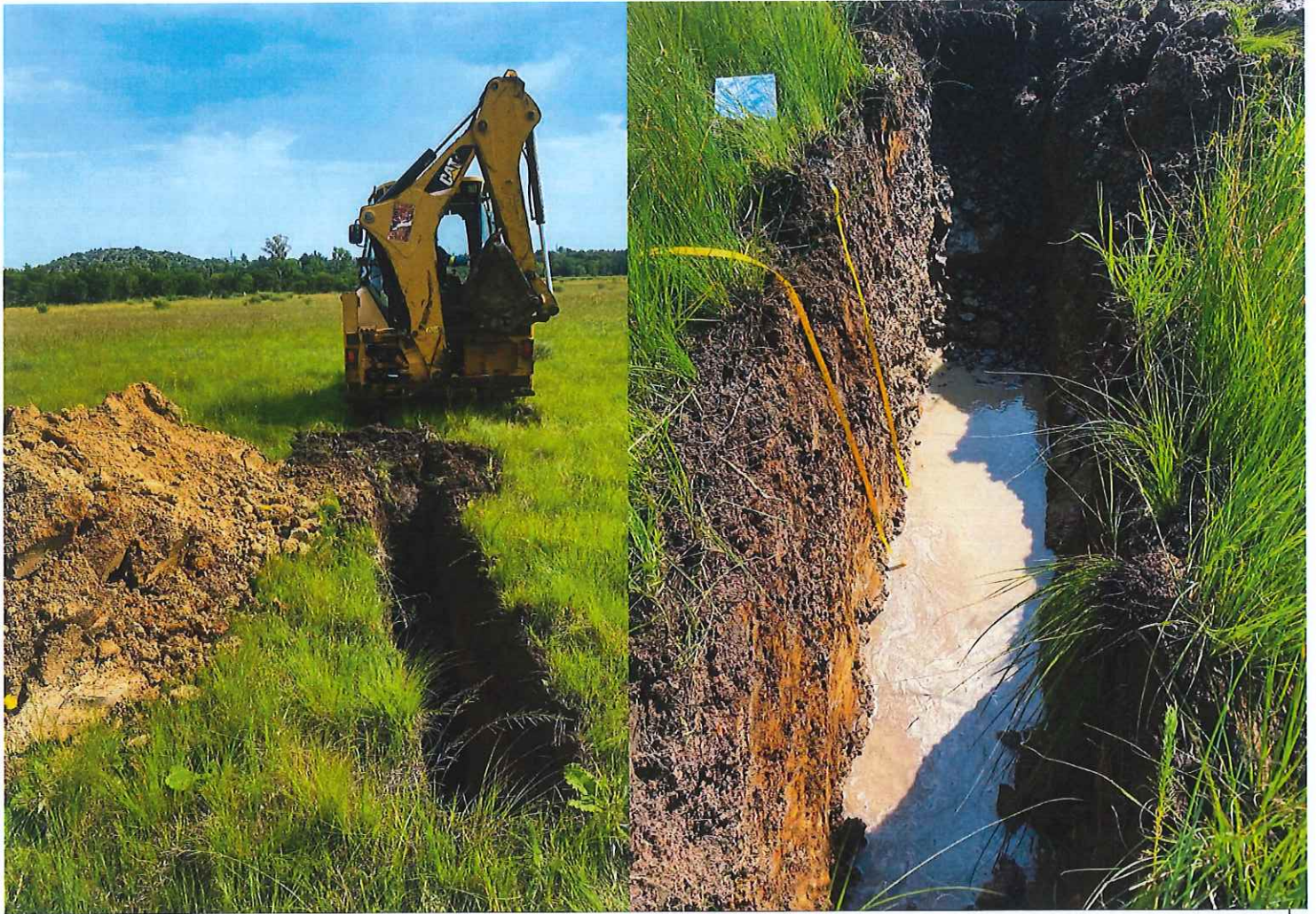
Digging of test hole TH01 and showing typical groundwater standing in test holes where encountered
