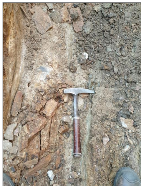
Note: TLB refusal in weathered gneiss.
