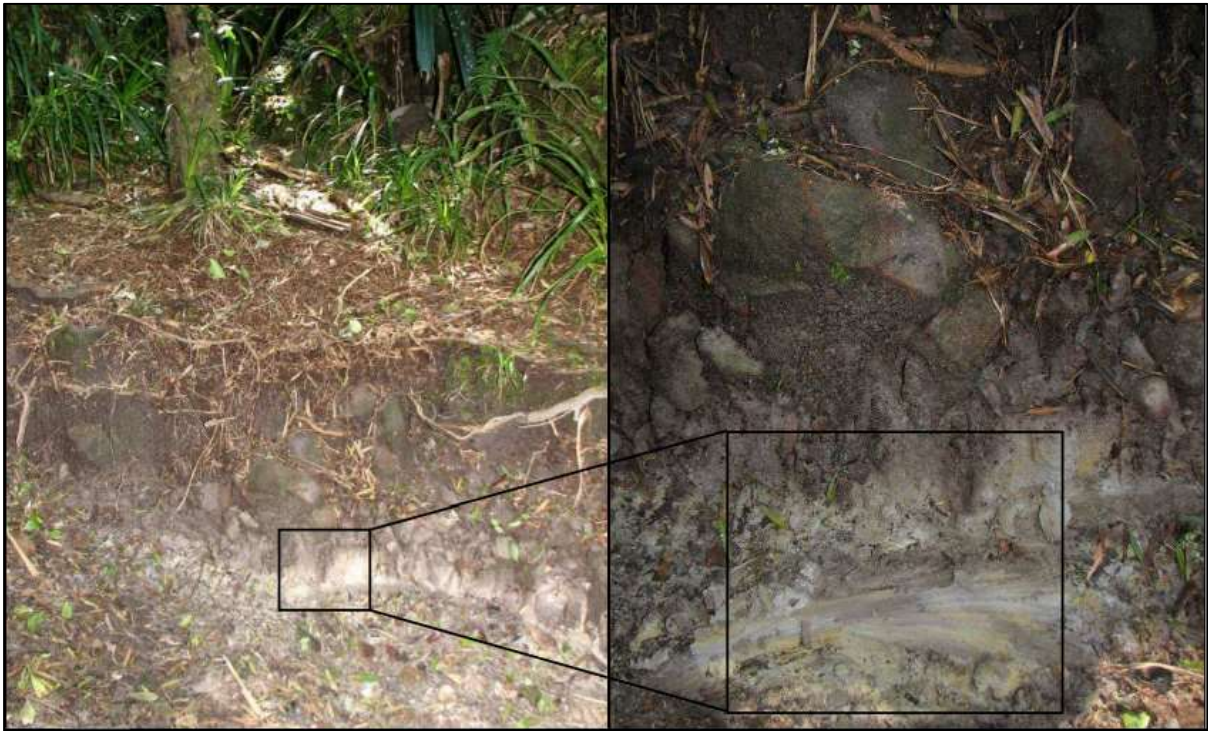
Figure 6: Gleyed saprolites (gley lithic horizon) observed upslope approximately 300m north of the proposed development
