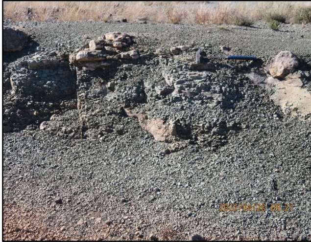
Photo 1: Lenses of slightly weathered fine grained sandstone (pinkish) in highly weathered siltstone (green) at position P4.
