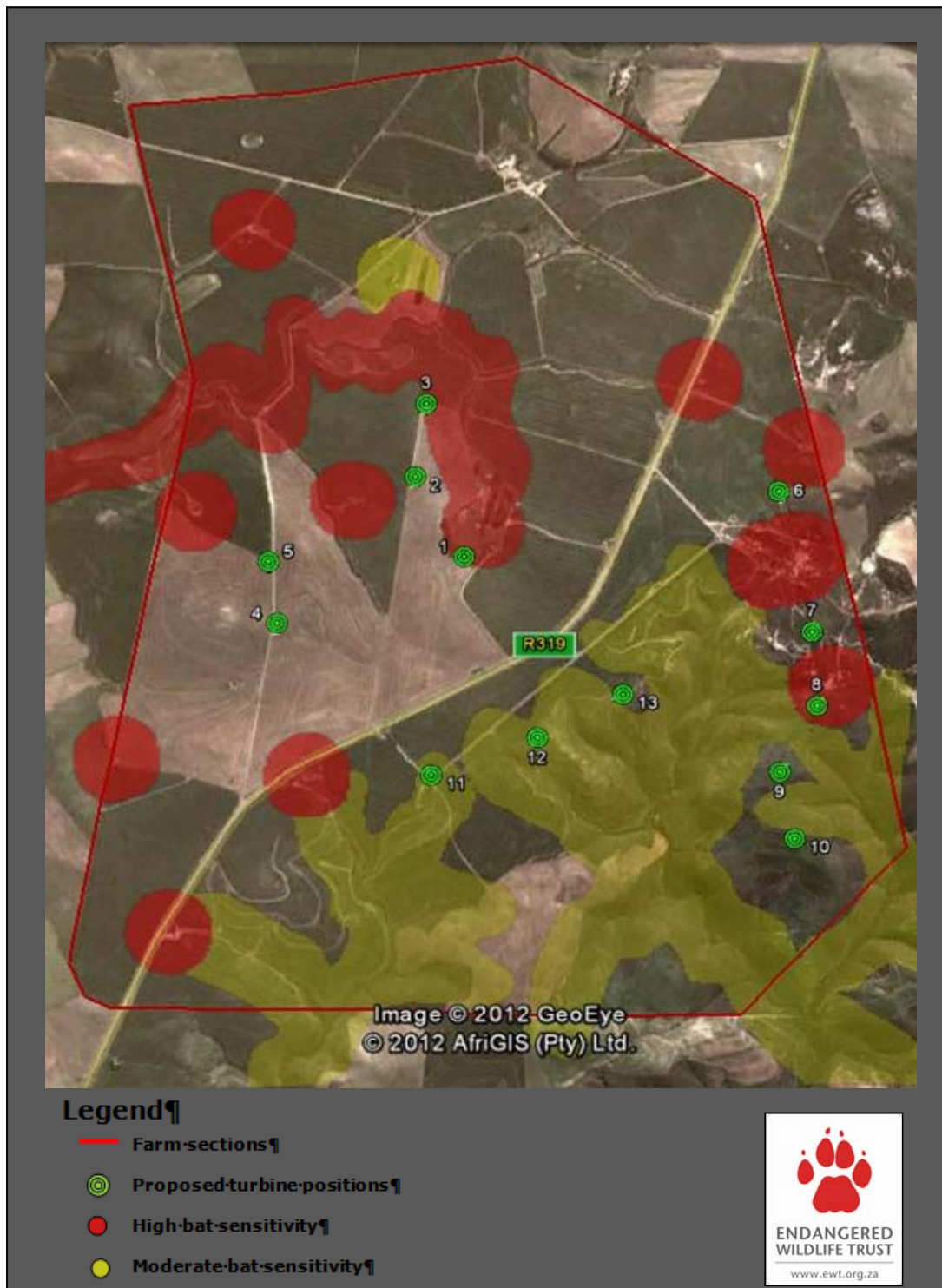
Figure 8.3: Bat sensitive habitats within the study area (as determined by the bat impact assessment) indicating the proposed layout
