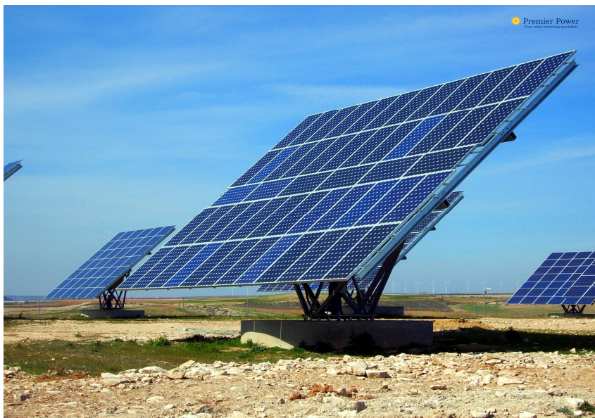
Figure 2.2: The support structures elevate the panels and allow for dual axis tracking of the sun for increased efficiency (Source: Gigaom)
