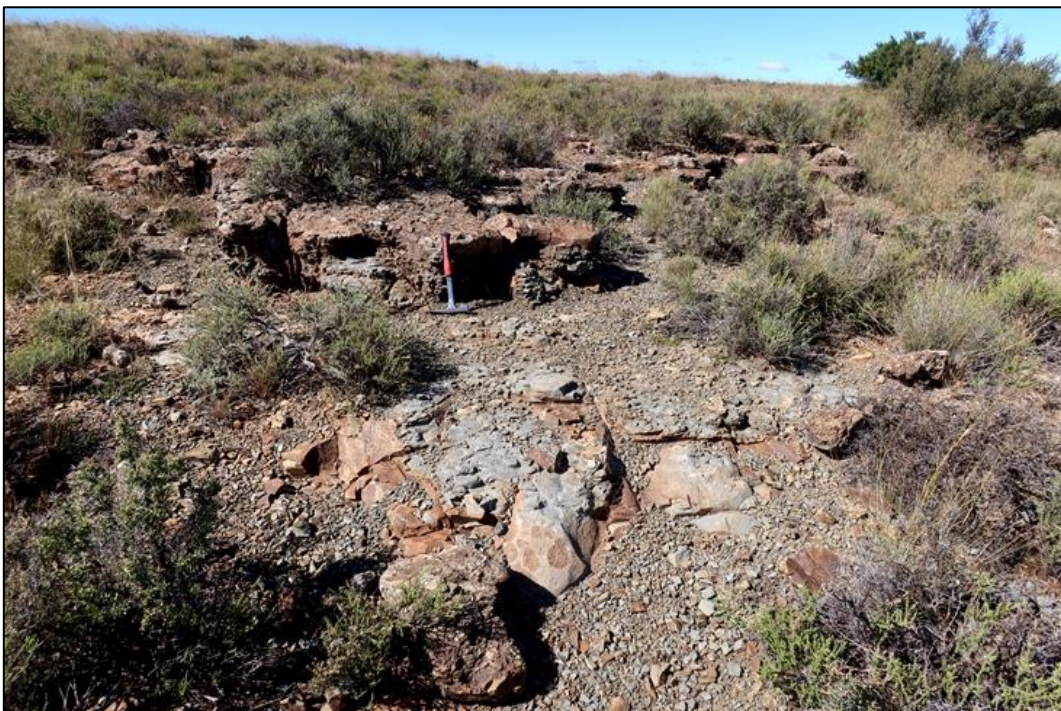
Figure 13: Prominent-weathering, thin horizon of pedogenic calcrete (possibly secondarily silicified), marked by hammer (30 cm long) within a baked overbank mudrock succession, eastern corner of Phase 3 Alt1b project area.
