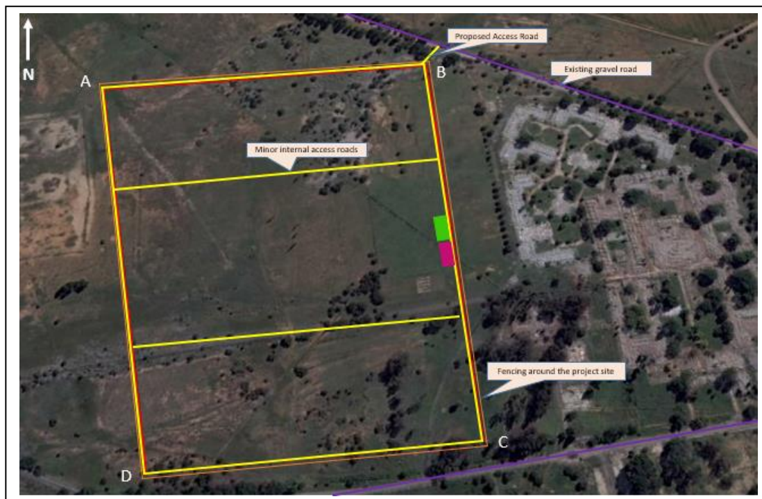
Figure 2: Map indicating access roads for the alternative site layout of the proposed PV Solar Facility
