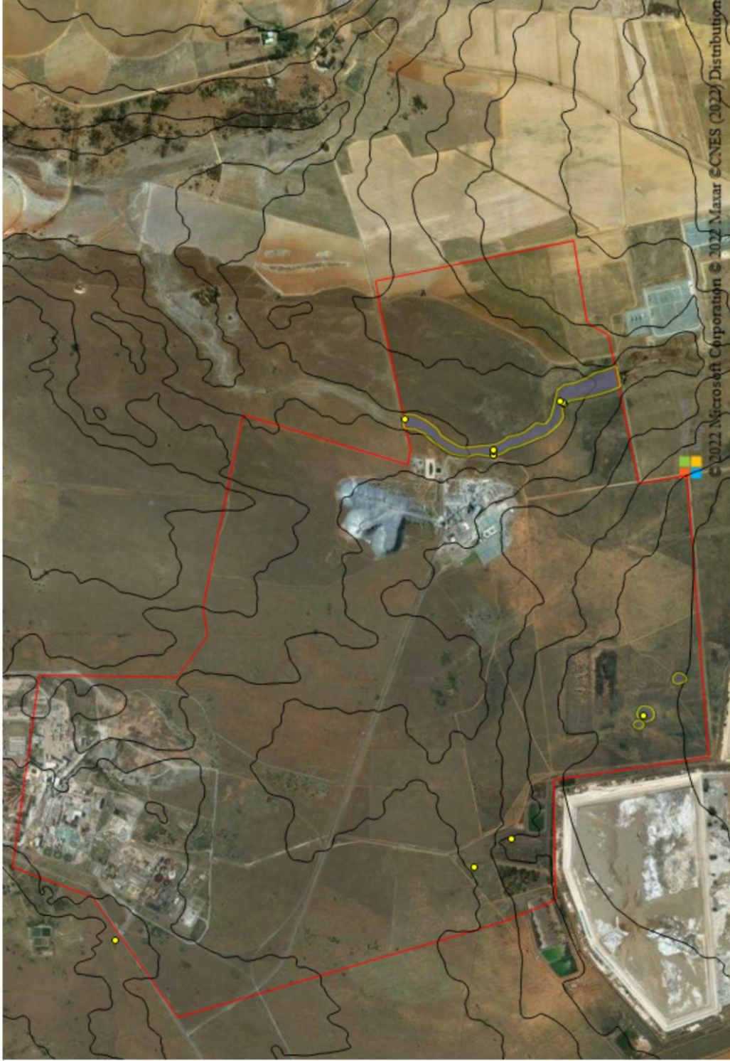
Map 3: Wetland delineation map of the proposed Harmony Moab-Noligwa Plant PV solar development near the town of Orkney. A large unchanneled valley bottom wetland system is situated in the eastern portion of the site and transects it from south to north. Three small depression wetlands are also located in the south west of the site. These wetland areas should all be excluded from the development and a 21 meter buffer also retained around them where the development occurs in close proximity. The wetland sampling points are also indicated.
