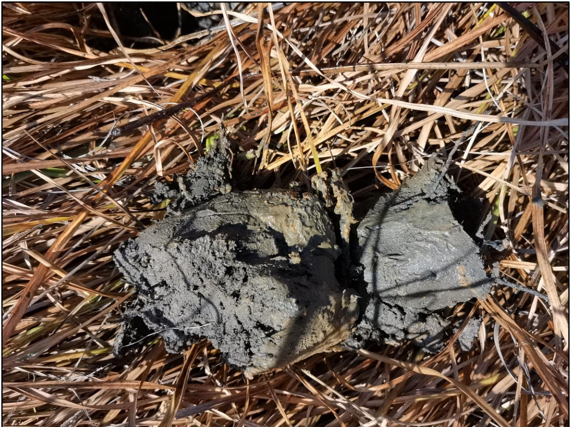
Figure 11 Example of the gley horizon of the Katspruit soil within the development area
