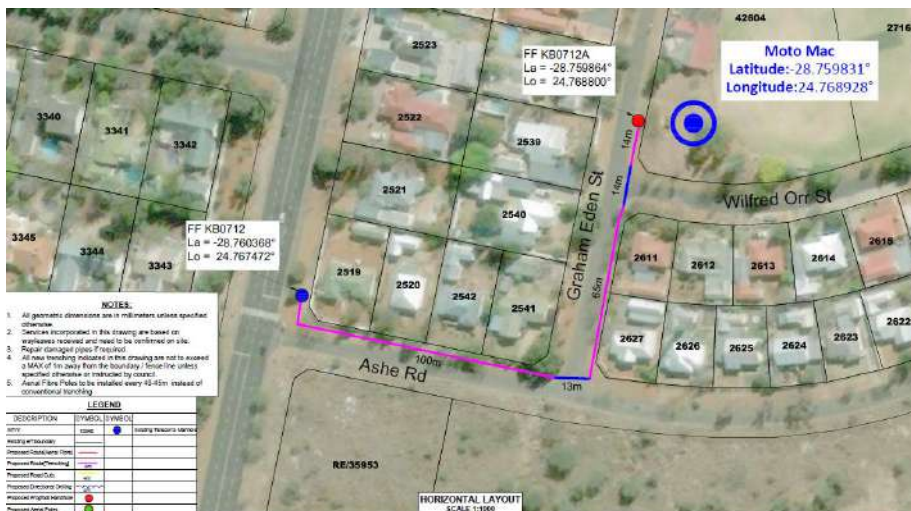
Figure 29: Section of optic fibre line connecting Moto Mac 5 G Rain Tower towards Oliver Road
