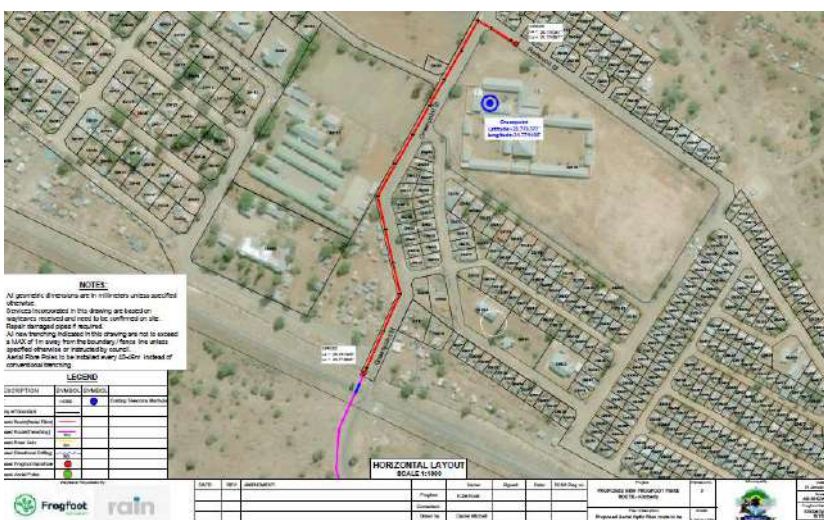
Figure 34: Optic fibre line connecting 5G tower at Green Point High School to Oliver Road
