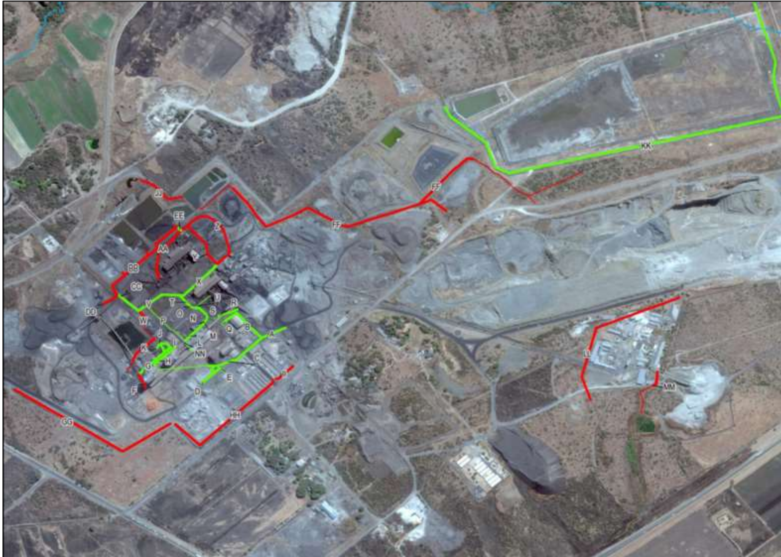
Figure 9.3.8.5(a): Current Storm Water Canals at HERNIC (Alloys Plant and Morula Mining)
