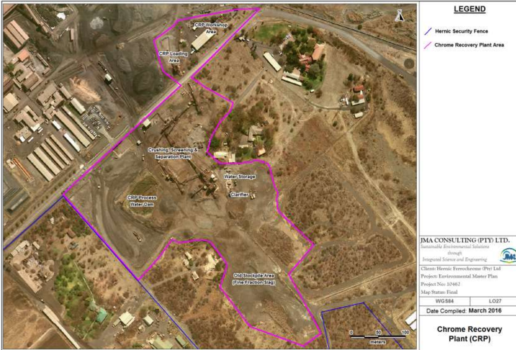
Figure 9.3.5.1(a): Location of and Infrastructure related to the Primary Chrome Recovery Plant (CRP)
