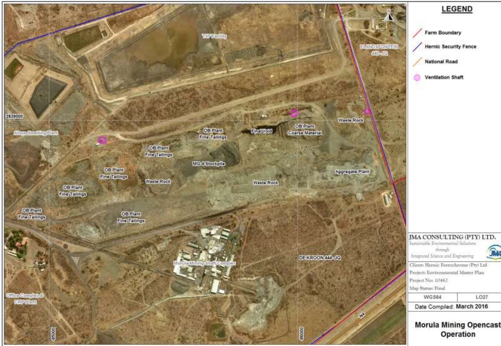
Figure 4.2.7.6(a): Location and Extent of Deposition of OB Plant Fines and Coarse Waste in the Morula Open Pit
