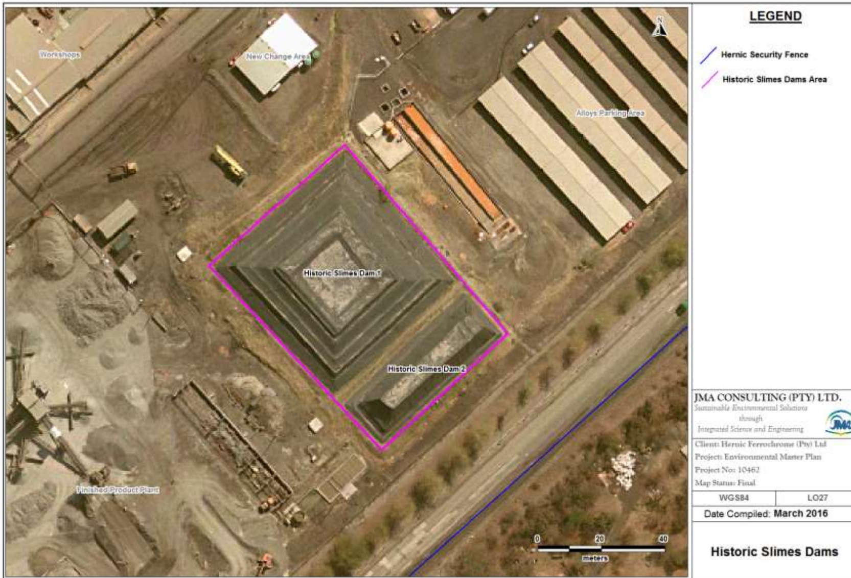
Figure 4.2.7.1(a): Location and Extent of the two Historic Slimes Dams
