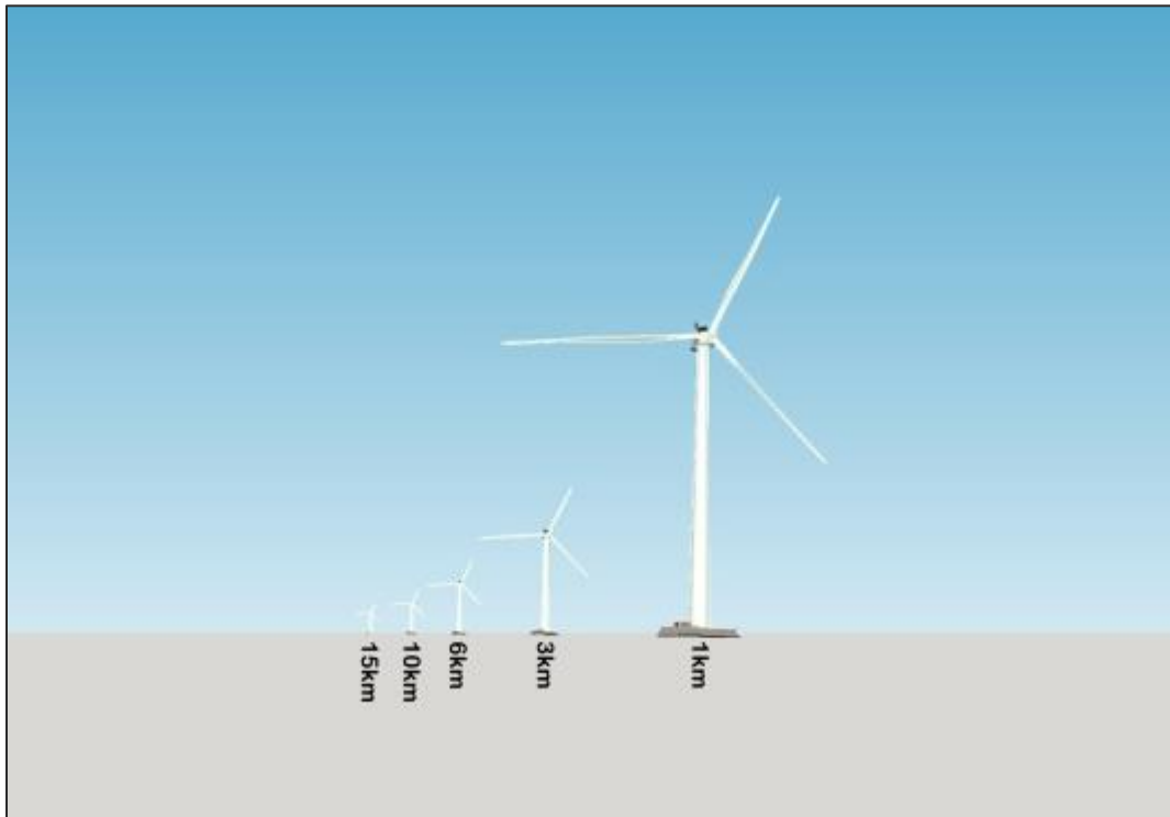
Figure 5: Conceptual representation of the diminishing visibility of a wind turbine over distance.
