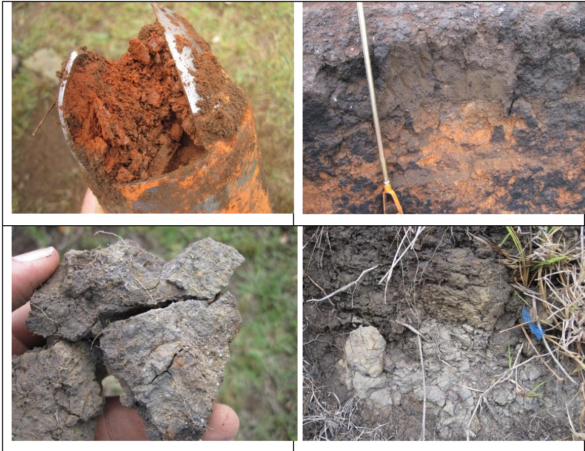
Figure 5: Illustrates a soil sample and profile within the study area that lack wetland indicators (top row); and a soil sample and profile that do contain signs of hydromorphism in the form of mottles in a low chroma(grey) matrix, sampled in the channelled valley bottom wetland (bottom row).
