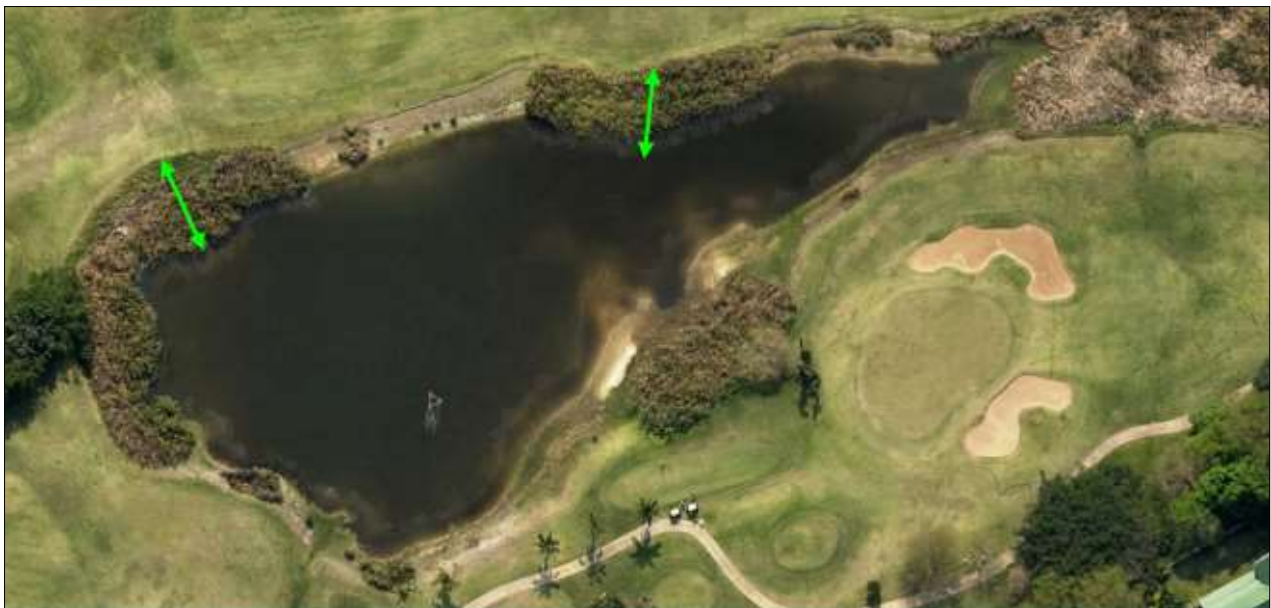
Figure 12: Image showing an example of a terraced dam edge which provides shallow flooding for the establishment of vegetation (Source: Kinvig and Associates Environmental Consulting).
