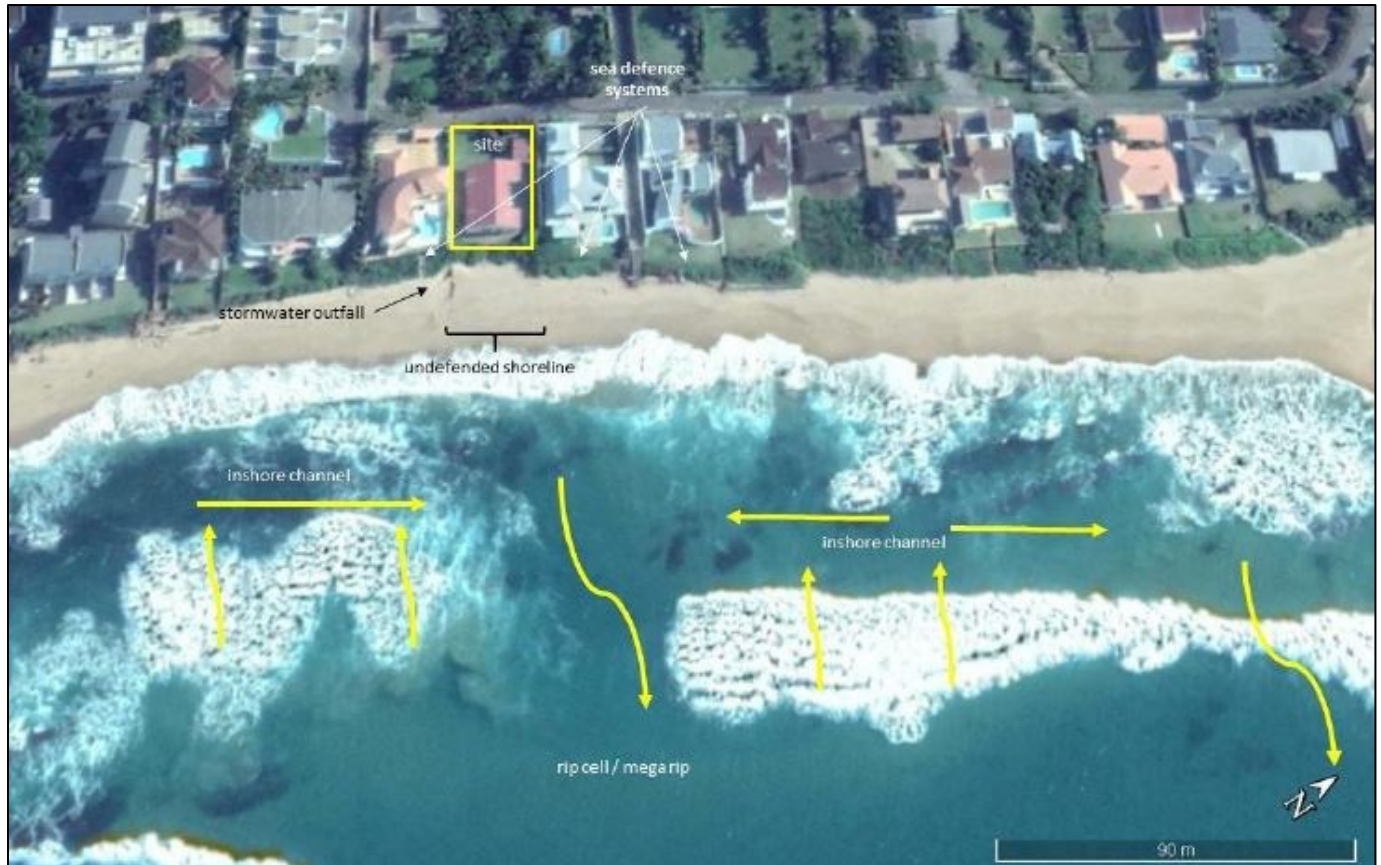
Figure 6: Aerial Photograph Showing Features and Coastal Dynamics Associated with House Gotz (Source: SDP, April 2021).
