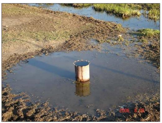
Plate 3: Artesian Borehole XBH 11
