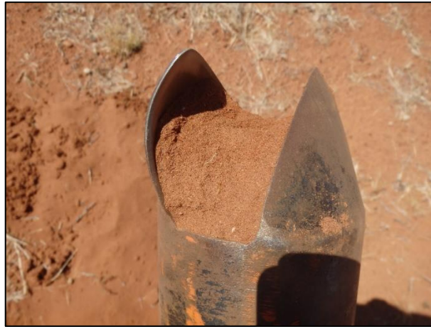
Figure 13: A representative example of a soil sample taken within the Vlermuisleegte River. This river has deep and sandy soils which are uniform in color throughout the 50cm sample pit taken.
