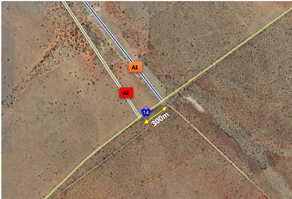
Figure 13: A2 Access Spacing
