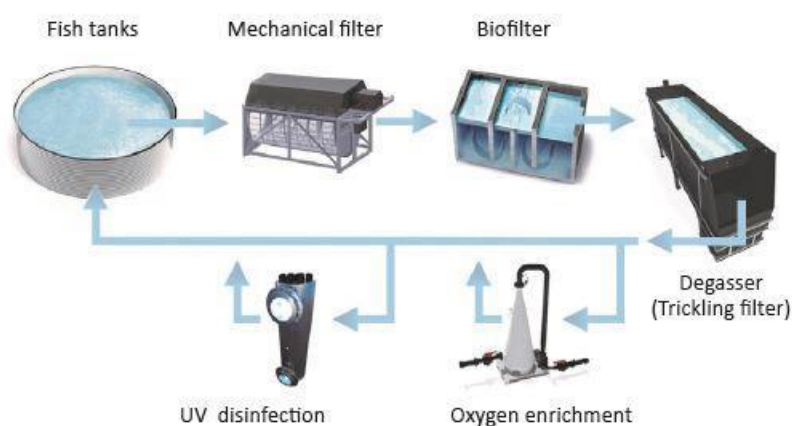
Figure 5: An illustration of the recirculating aquaculture system aquaponics
