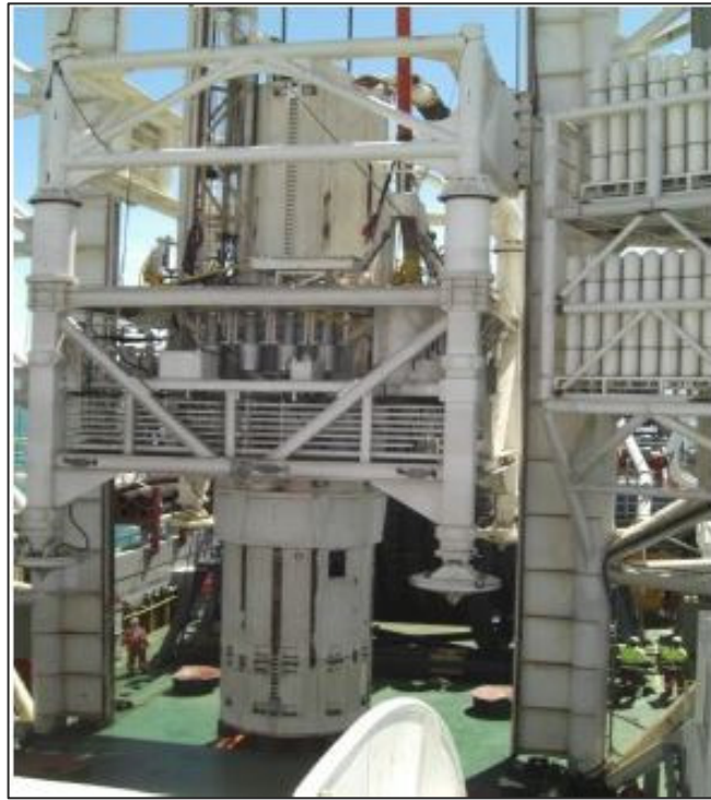
FIGURE 3-5: THE 2.5 M DIAMETER DRILL BIT WITHIN THE DRILL FRAME STRUCTURE.
