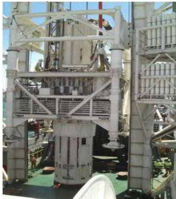
Figure 4: The 2.5 m diameter drill bit within the drill frame structure.
