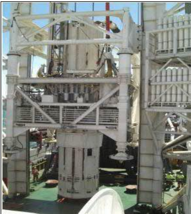
Figure 3-3: The 2.5 m diameter drill bit within the drill frame structure.
