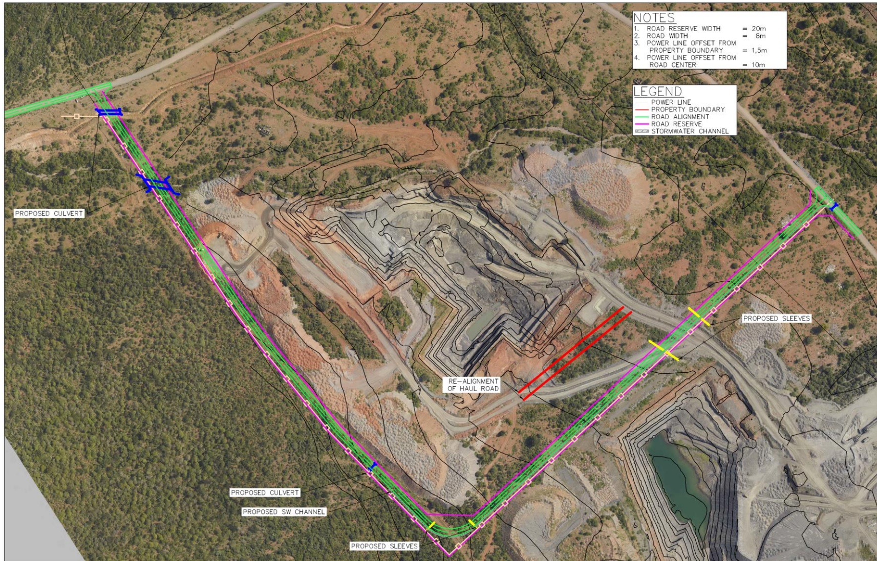
Figure 3: Layout map of the proposed D4134 road (Preferred option) and 22 kV powerline relocation including additional stormwater management infrastructure
