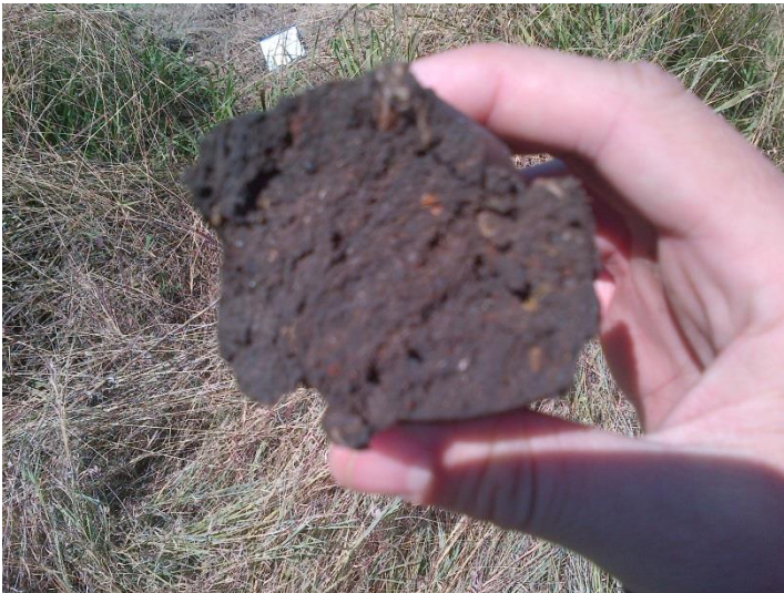
Photo 2: Redoximorphic features indicative of wetland soils evident in the soil samples.
