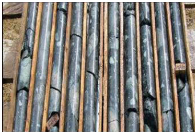
Plate 2: Geological Core Samples from Prospecting Drilling
