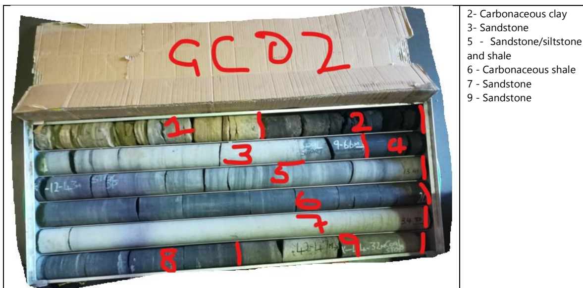
FIGURE 31-2: ANNOTATED PHOTOGRAPH OF DRILL CORES OF A SAMPLE OF OVERBURDEN MATERIAL
