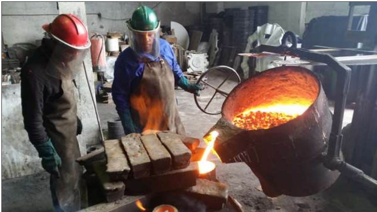
Figure 5: Pouring molten metal
