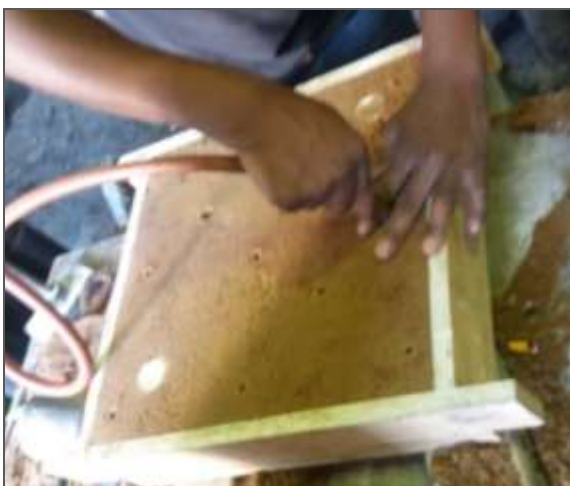
Figure 3: Pumping CO 2 gas into the mould until it hardens
