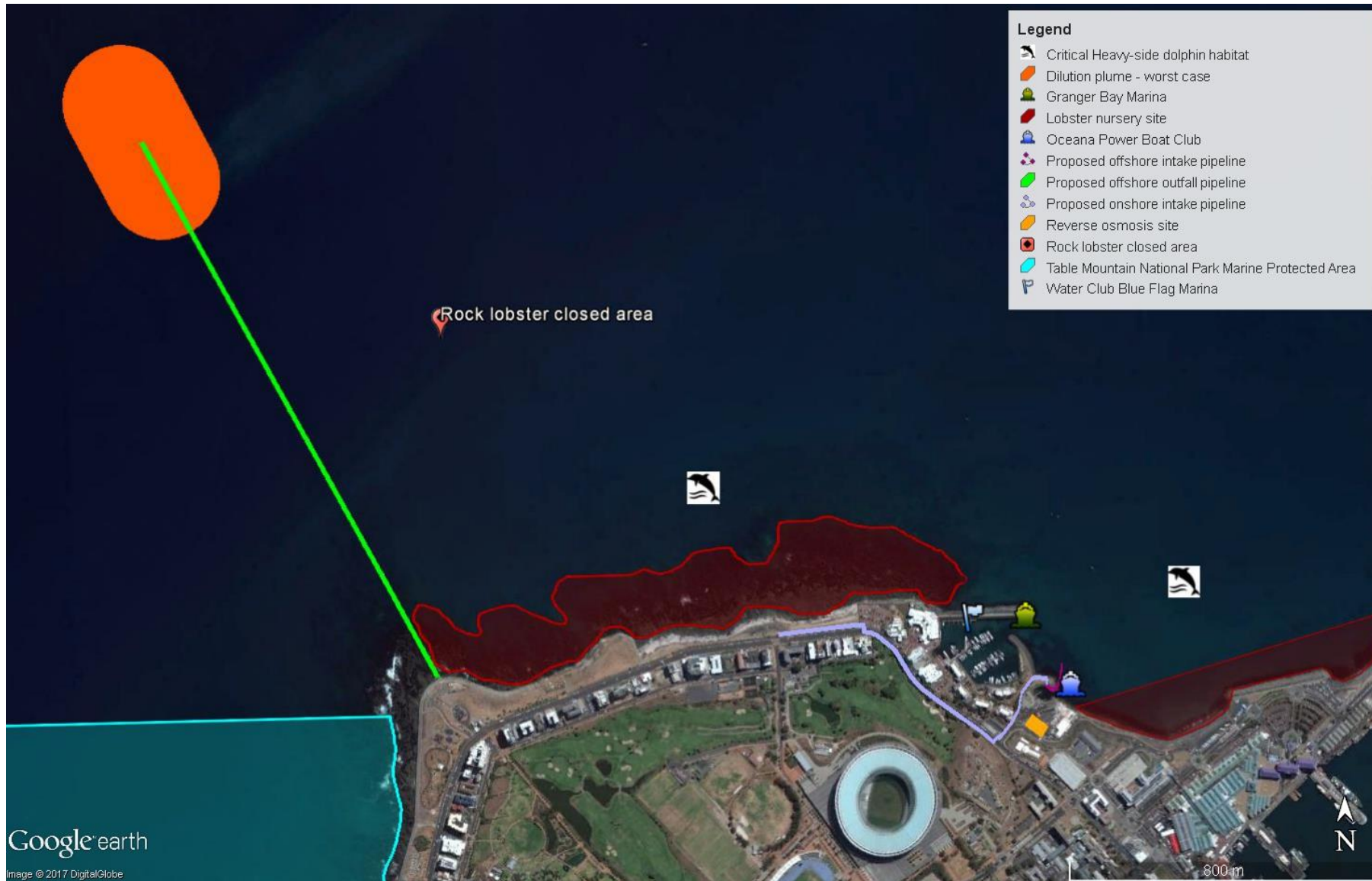
Figure 3.8 Sensitivity map for Granger Bay showing proposed pipeline locations and sensitive environments (Google Earth 2017).
