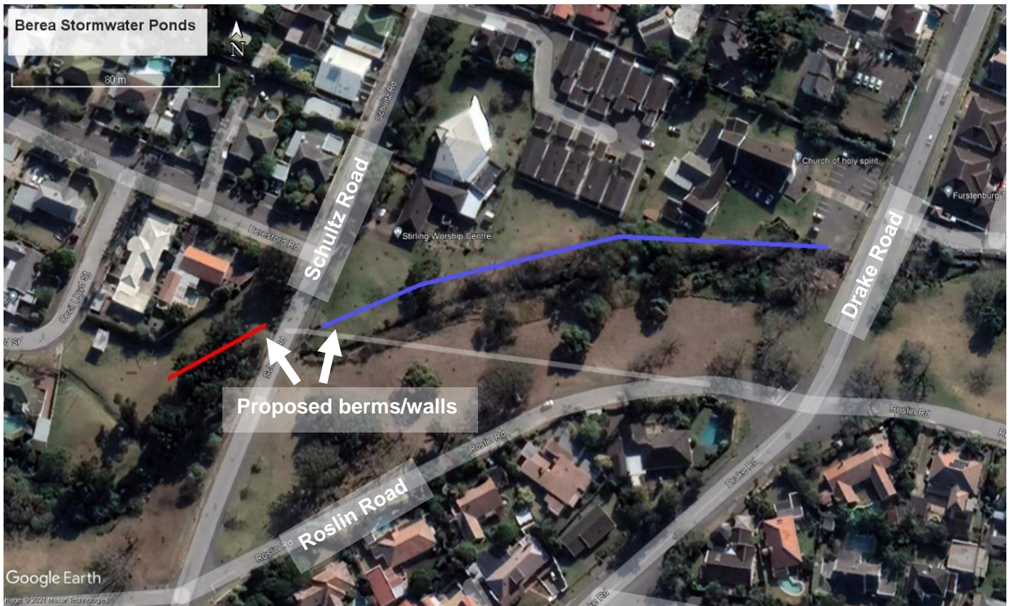
FIGURE 2: Location of the proposed grass-lined earth berms / gabion basket walls adjacent to Schultz and Drake Road in Stirling.
