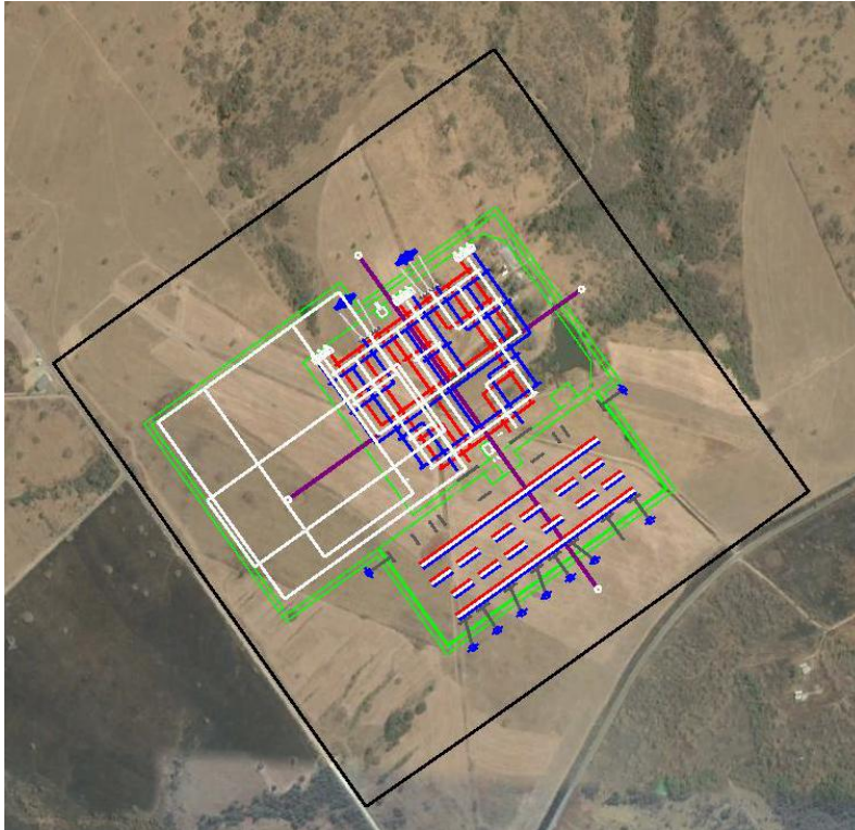
Figure 7 Layout 1: 400 kV yard facing the road and space for future lines on the west
