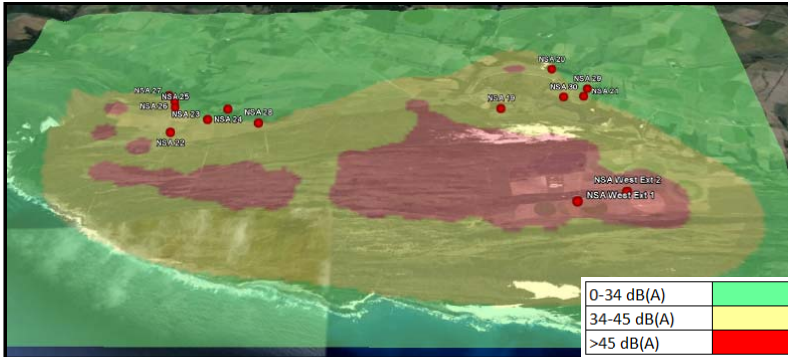
Figure 19 - Raster Image of Western Site Isopleths & NSA's (Nordex N90 -Wind speed 8m/s)
