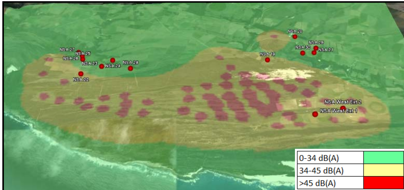
Figure 18 - Raster Image of Western Site Isoleths & NSA's (Nordex N90 -Wind speed 4m/s)
