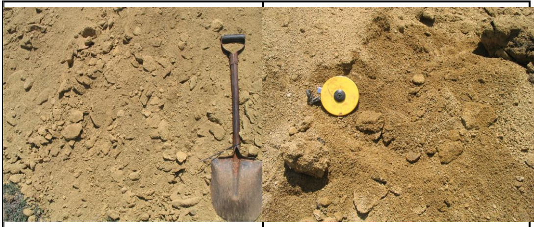
Figure 5.4.4 (a): Images of Friable “Sugar” Dolerite
