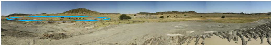
Figure 14: Panorama of the mine sump situated to the south of the processing plant. This is the same dump as depicted in Fig. 1 which obstructs a drainage line and leads to the formation of an artificial wetland (blue figure).
