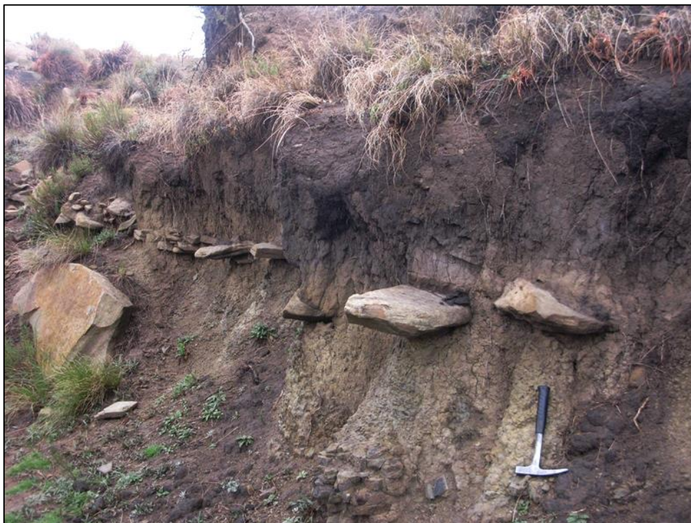
Fig. 25. Sandy soils with well-developed stone line overlying weathered Katberg mudrocks and overlain in turn by dark grey modern carbonaceous soils, Farm RE13 (Loc. 037) (Hammer = 27 cm).
