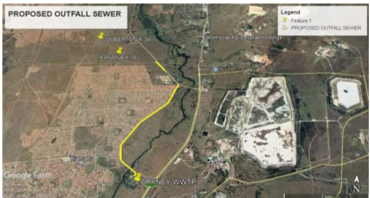
Figure 14: Proposed route of outfall sewer line
