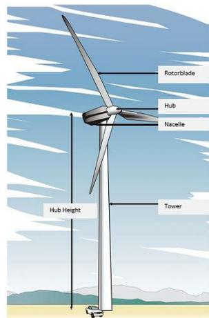
**Figure 1-3** Main components of a wind turbine
