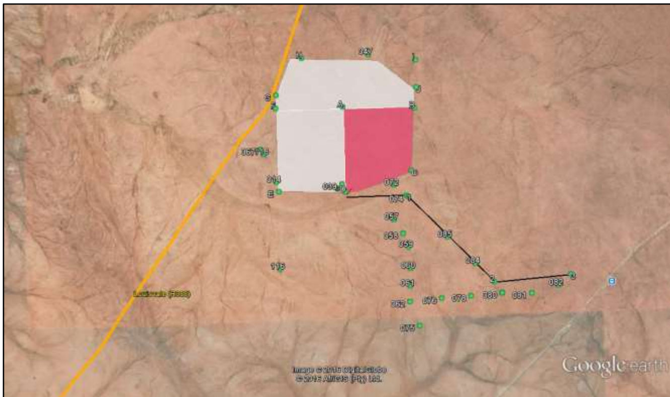
Figure 18: Showing soil sample points undertaken along the proposed overhead powerline to the Niewehoop powerstation.
