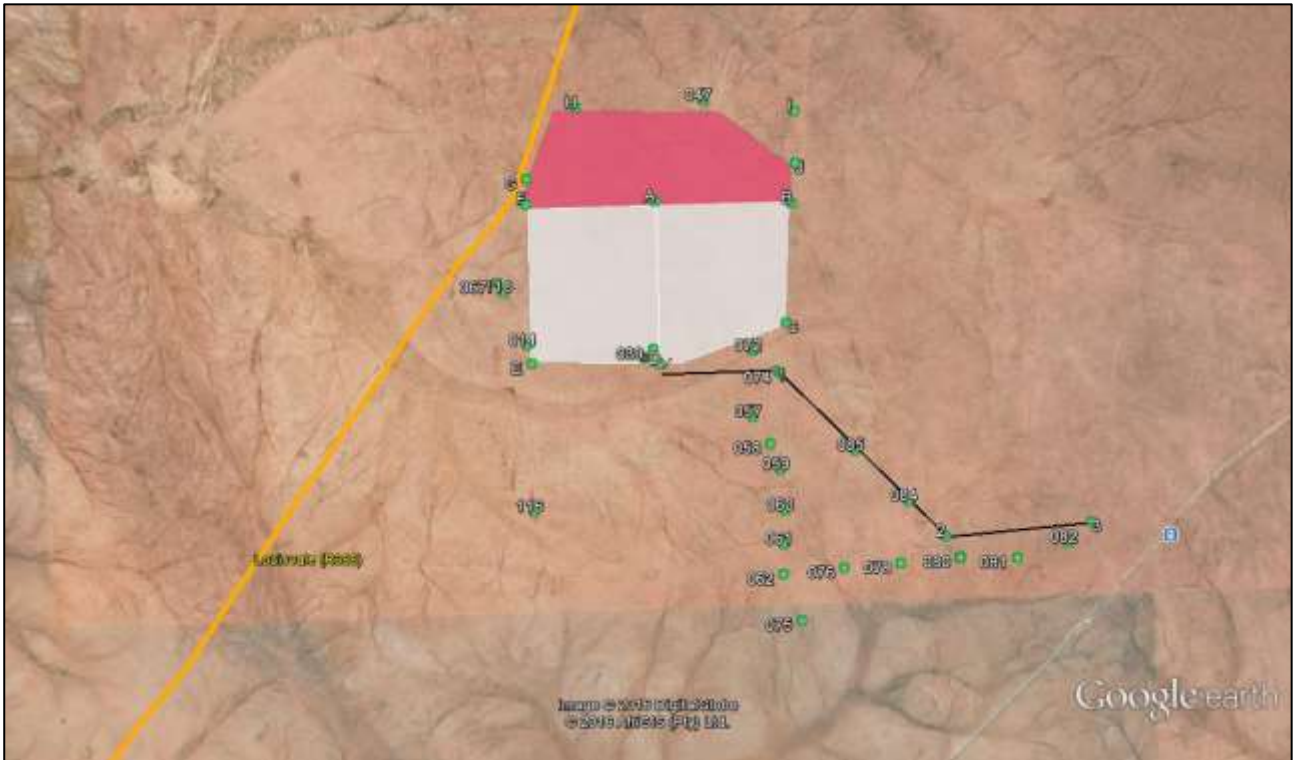
Figure 18: Showing soil sample points undertaken along the proposed overhead powerline to the Niewehoop powerstation.
