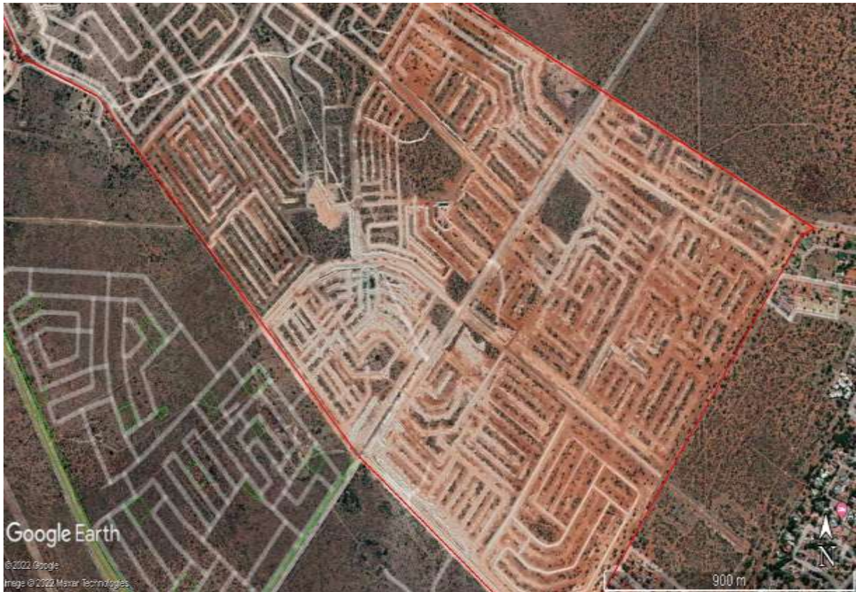
Figure 3: A closer view of the study & development area in March 2022 showing the extent of the earthworks related to the installation of services (sewerage, water pipelines & internal road networks (Google Earth 2022).
