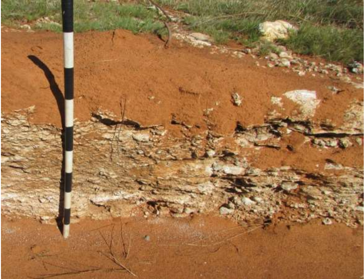
Figure 17: The layer of red sands overlaying the calcrete is clearly visible here.
