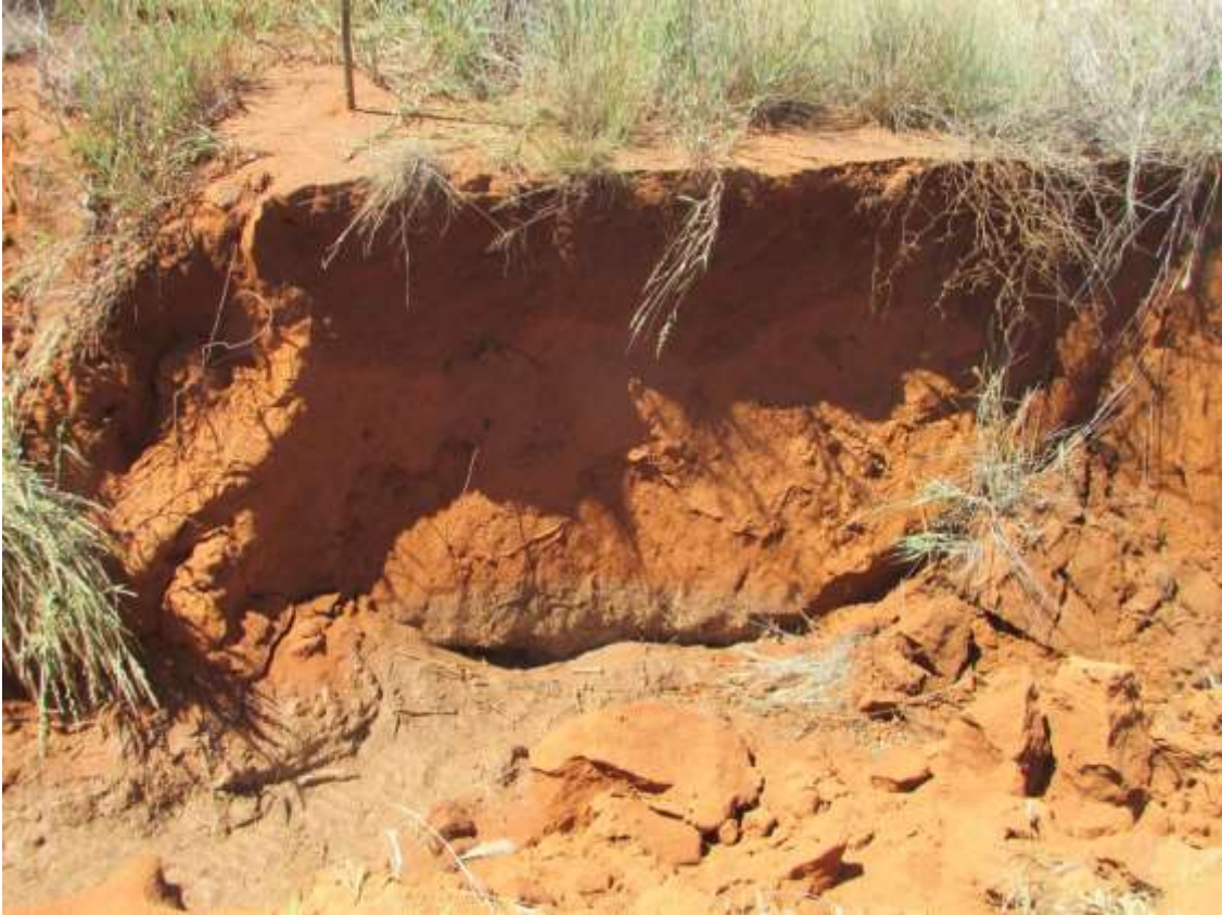
Figure 16: In some areas the red Aeolian (Kalahari) sand layer is up to 1.50m thick.
