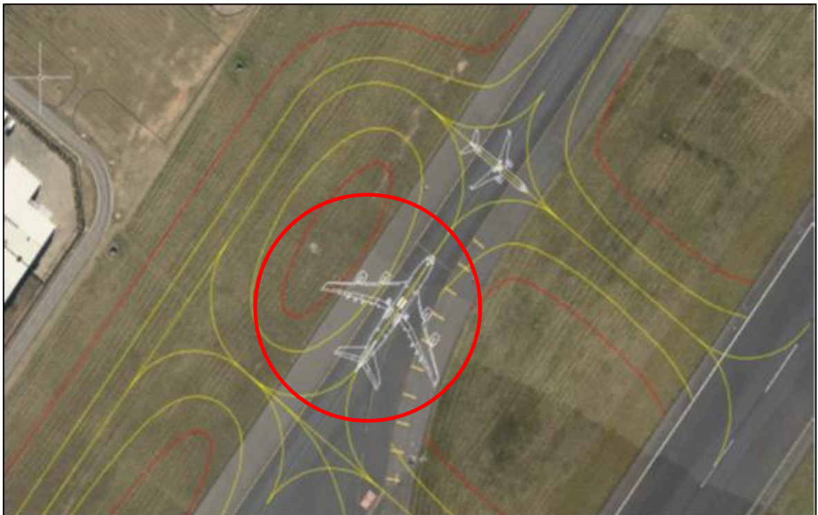
Figure 11: Option 2 intersection taxiway north of RET
