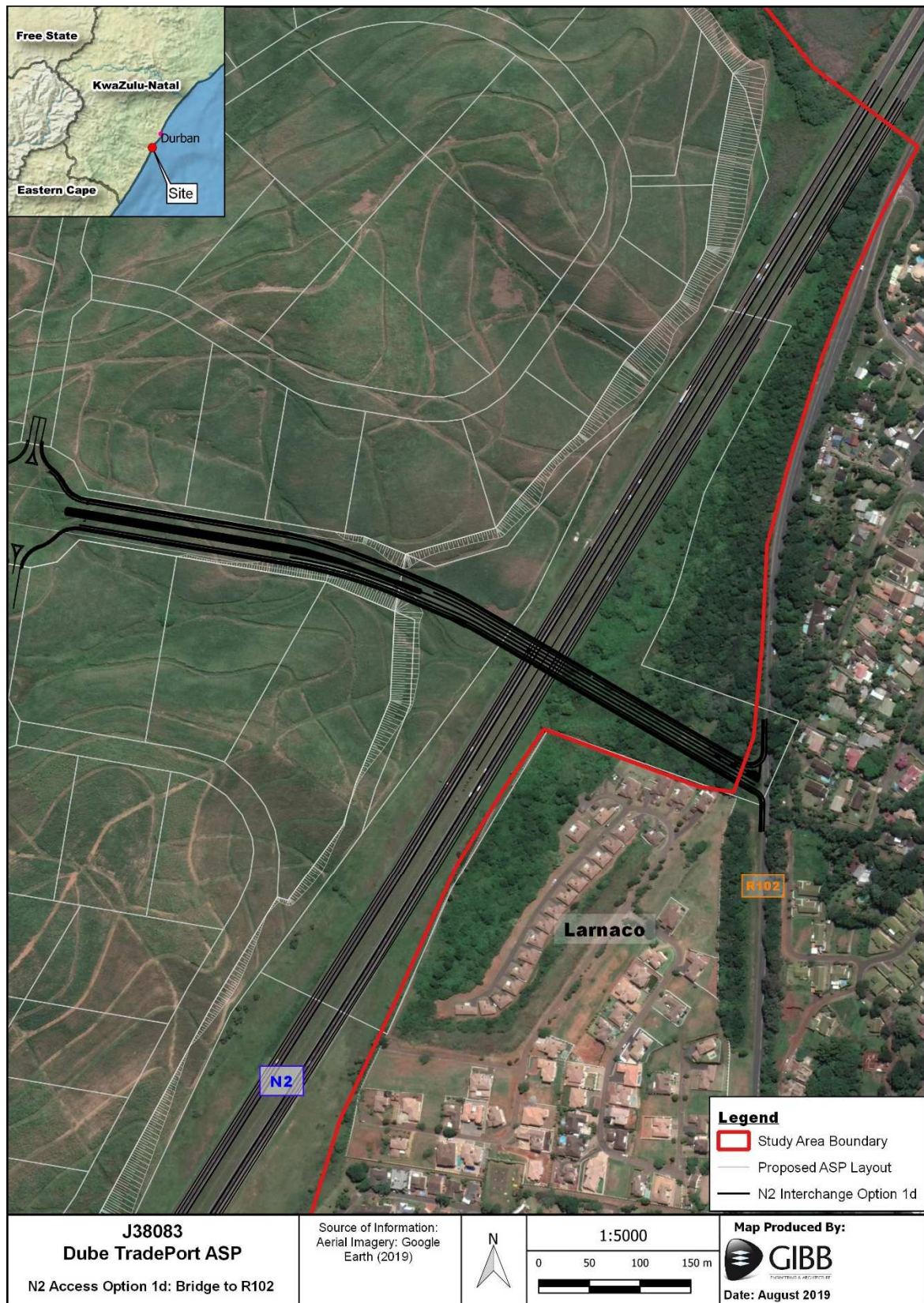
Figure 2-10: Option 1D: A new bridge from the R102 with no access off the N2
