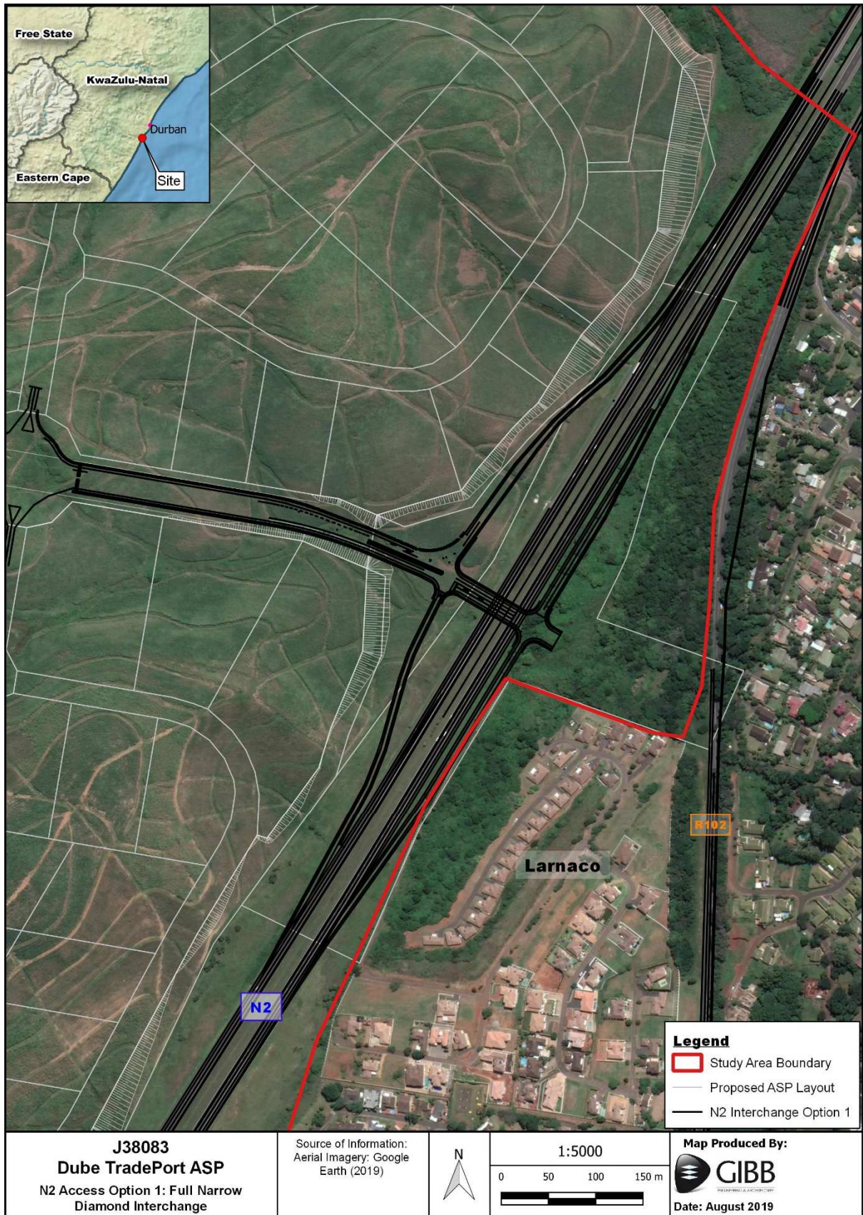
Figure 2-8: Option 1: New Narrow Diamond Interchange of the N2 with no link bridge to the R102
