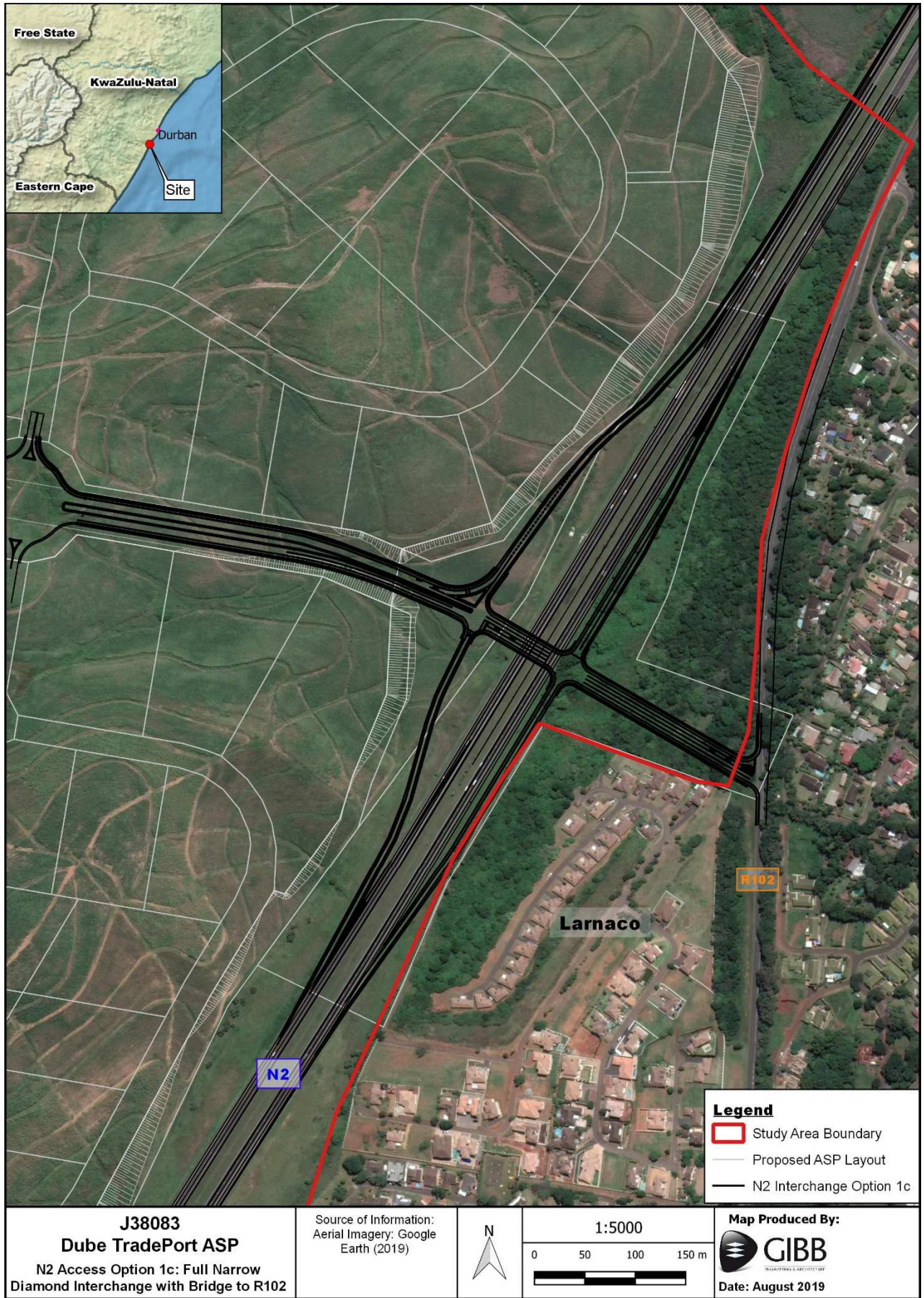
Figure 2-9: Option 1C: Narrow diamond interchange of the N2 with a new link to the R102
