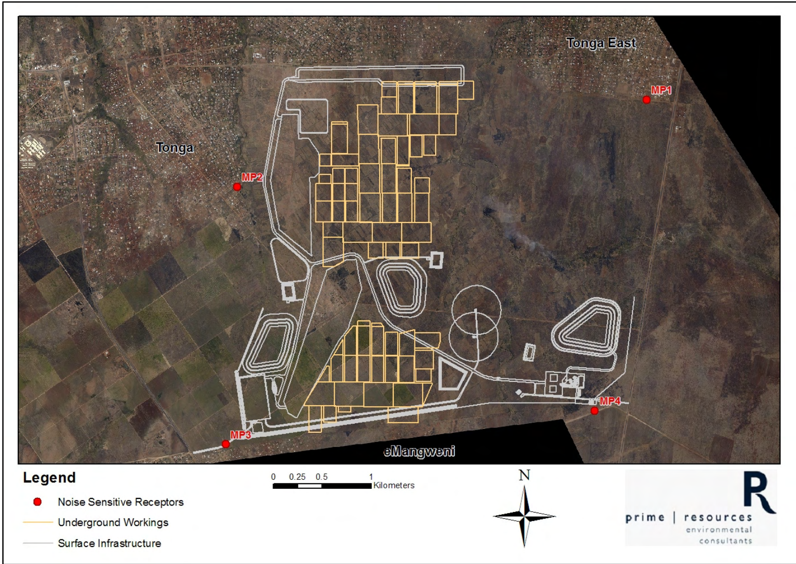
Figure 33: Baseline noise monitoring points representative of noise sensitive receptors.
