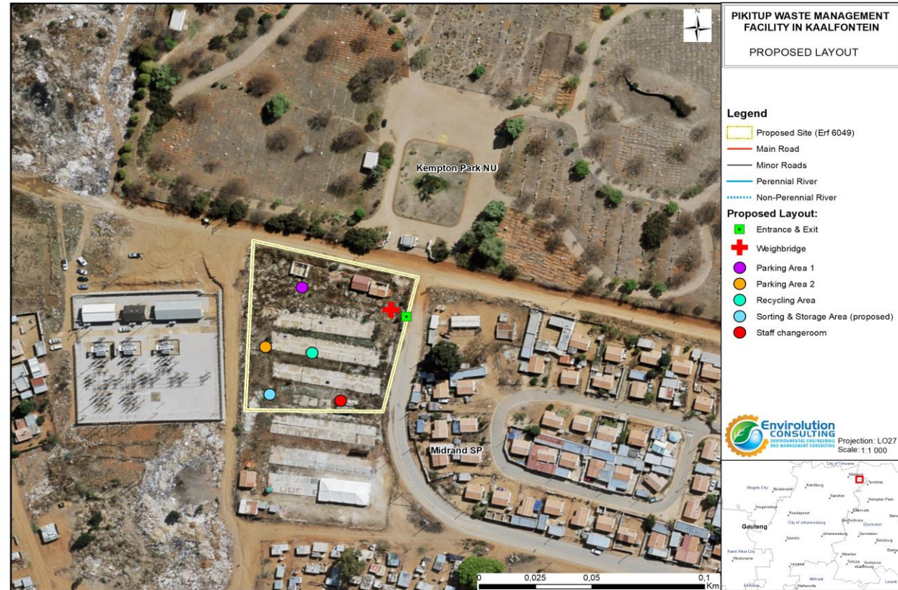
Figure 1: The proposed (preferred) layout of the waste facility (Sorting and Storage Area on the South West corner ).
