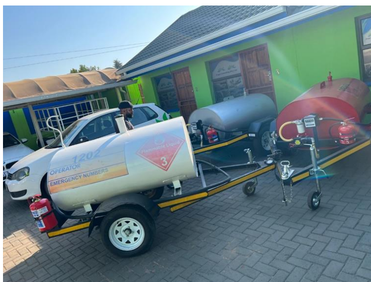
Figure 5: Typical example of mobile fuel storage. [ Singo Consulting,2023]
