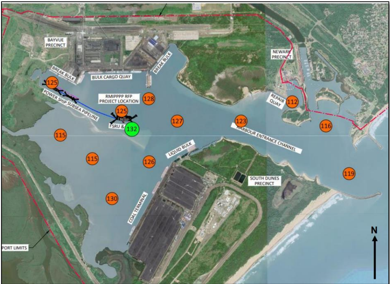
Figure 6-28: Average dB SPLRMS baseline levels from attended measurements in Port of Richard’s Bay between 15th and 17th November 2021 (including proposed location of the Powerships)
