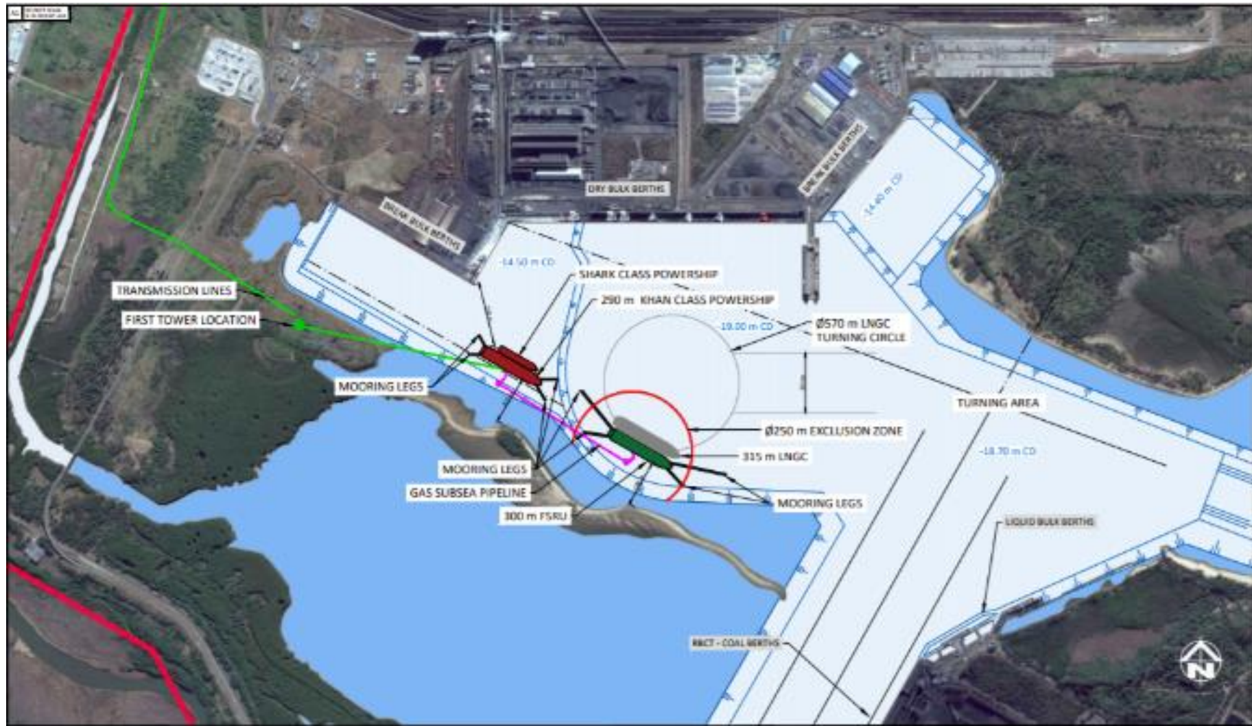
Figure 3-5: Alternative 2: Powerships and FSRU position within the port – further from transmission tower.
