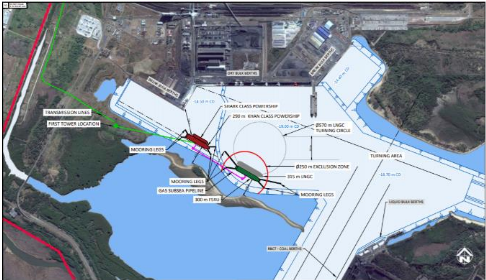
Figure 3-7: Alternative 2: Gas Pipeline route (Pink Line)
